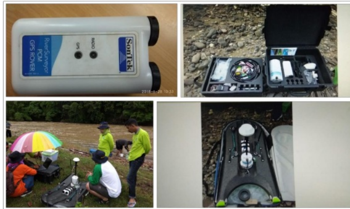
Figure 2. Tools used Acoustic Doppler Current Profiler (ADCP) Sontek Hydro Surveyor.
